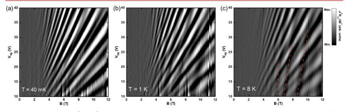
**Figure 2.** Color mapping of  $-\partial^2 R_{xx}/\partial B^2$  by changing the back gate voltage  $V_{bg}$  and magnetic field *B* under various temperatures of 40 mK (a), 1 K (b), and 8 K (c). Top gate voltage  $V_{tg}$  is fixed at 0 V.
